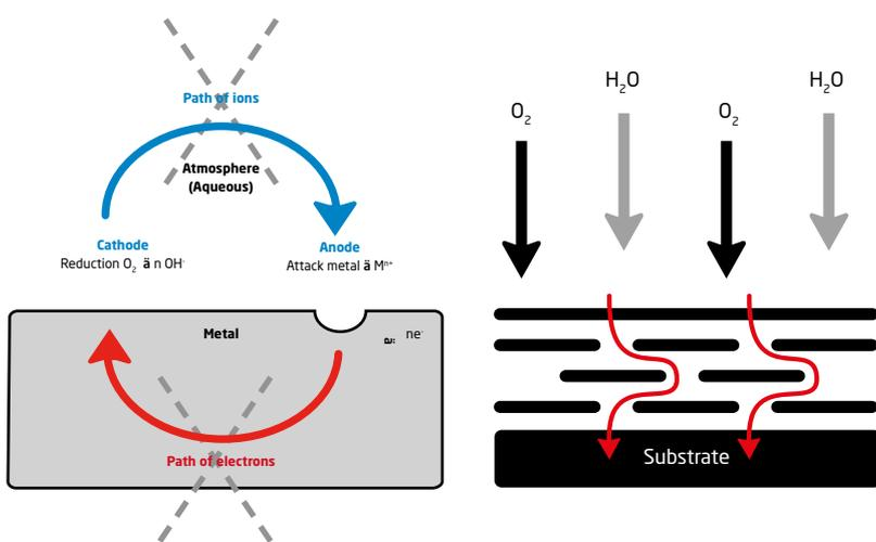
Corrosion is an electrochemical process consisting of cathodic and anodic reactions fed by electrons and ionic diffusion. Alesta® ZeroZinc anticorrosion primers work by preventing at least one of these reactions.
